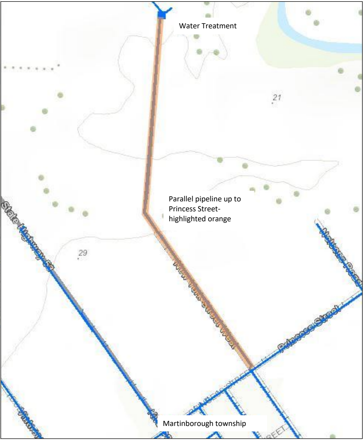
Pictorial of Water treatment plant to Princess St
